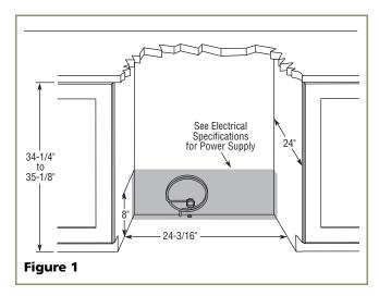
Follow the cut-out drawing in **Figure 1**. The 24-3/16" width allows 1/4" for ease in installation and removal of the unit. The 24" depth is the counter depth in most installations. The unit is 24" deep including the handle on Black and White models and 24" deep including the door and *not* the handle on Stainless Steel models (see **Figure 2**).
